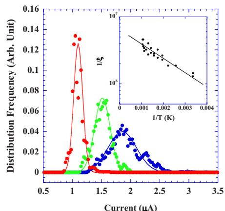
FIG. 3. (Color online) Histogram of the emission-current intensity at 300 K (rightmost, blue circles), 700 K (center, green circles), and 925 K (leftmost, red circles) in a  $\text{H}_2$  atmosphere; the solid lines are the theoretically fitted curves. The inverse of the variance,  $1/\xi$ , for each temperature obtained by the theoretical fitting is shown as solid circles. The solid line is the fitted curve with a physical adsorption energy of 45 meV.
