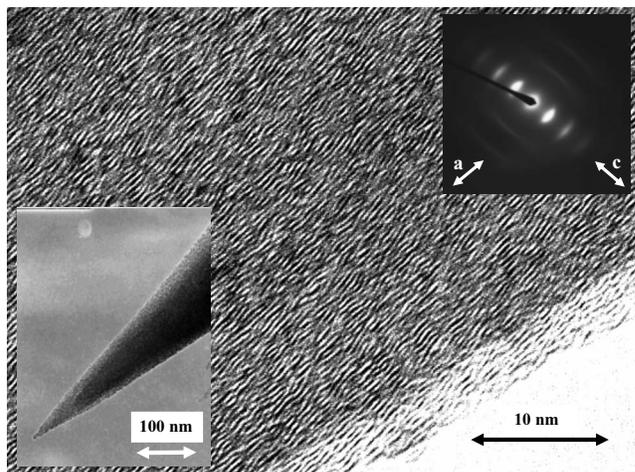
FIG. 1. TEM image (left inset), HRTEM image, and the selected area electron diffraction pattern (right inset) of a single graphene nanoneedle.
