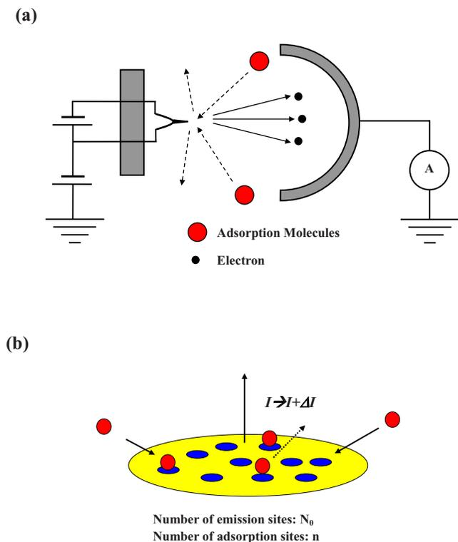
FIG. 2. (Color online) (a) Schematic diagram of the system used to measure fluctuation of the field emission current as a function of cathode temperature in the presence of various purified gases. (b) Physical desorption model in which fluctuation of the emission current originates from the adsorption and desorption of molecules onto the emission sites.
