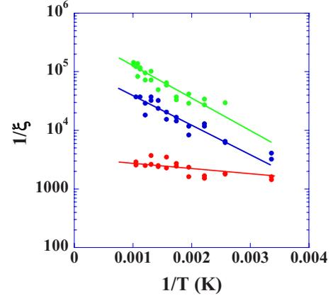
FIG. 4. (Color online) Inverse of the variance,  $1/\xi$ , for CO molecules (top, green circles), Ar molecules (center, blue circles), and He molecules (bottom, red circles) as a function of GRANN cathode temperature. The solid lines are the fitted curves with physical adsorption energies of 110 meV for CO molecules, 100 meV for Ar, and 15 meV for He.
